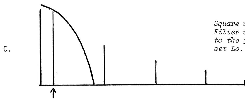
Square wave into a Low Pass Filter with the Filter "tuned" to the fundamental, Resonance set Lo.
