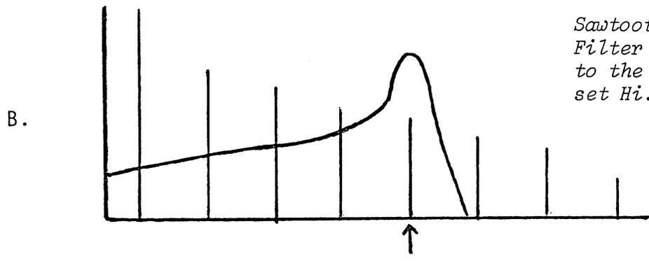
Sawtooth wave into a Low Pass Filter with the Filter "tuned" to the 5th harmonic, Resonance set Hi.
