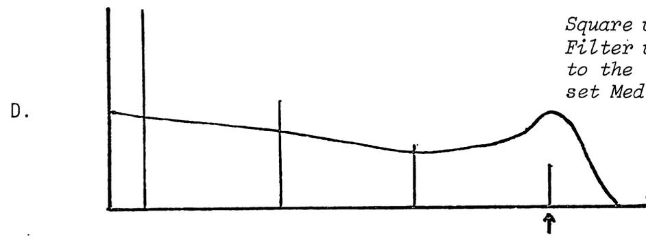
Square wave into a Low Pass Filter with the Filter "tuned" to the 7th harmonic, Resonance set Med.
