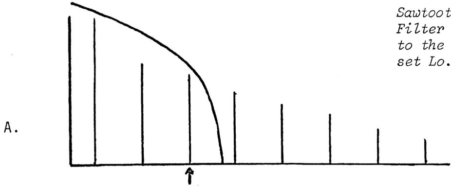
Sawtooth wave into a Low Pass Filter with the Filter "tuned" to the 3rd harmonic, Resonance set Lo.
