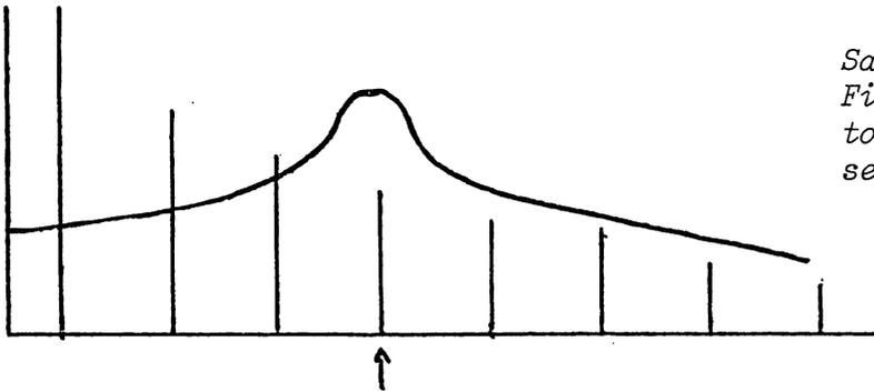
*Sawtooth wave into a Band Pass Filter with the Filter "tuned" to the 4th harmonic, Resonance set Med.*
