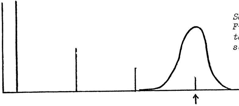
*Square wave into a Band Pass Filter with the Filter "tuned" to the 7th harmonic, Resonance set Hi.*
